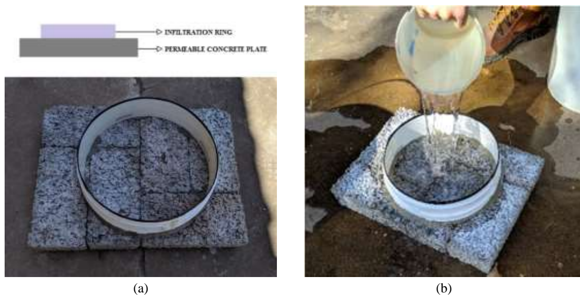
Figure 4: (a) Representative scheme and configuration of the materials used in the permeability test; (b) Pre-wetting of permeable concrete plate.
